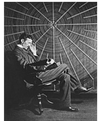
Tesla sitting in front of a spiral coil used in his wireless power experiments at his East Houston St. laboratory
